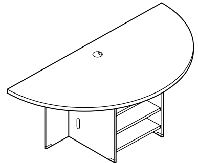
TC 266 (Desk Top) Team Computer Workstation 1800 x 900 x 675 mm 71" x 35 1 / 2 " x 26 5 / 8 " inch
